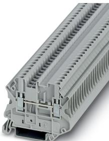
Feed-through terminal block, nom. voltage: 800 V, nominal current: 24 A, connection method: Screw connection, number of connections: 2, number of positions: 1, cross section: 0.14 mm<sup>2</sup> - 4 mm<sup>2</sup>, AWG: 26 - 12, width: 5.2 mm, color: gray, mounting type: NS 35/7,5, NS 35/15
