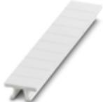
Zack marker strip, Strip, white, unlabeled, can be labeled with: PLOTMARK, CMS-P1-PLOTTER, mounting type: snap into tall marker groove, for terminal block width: 5.2 mm, lettering field size: 5.1 x 10.5 mm, Number of individual labels: 10
